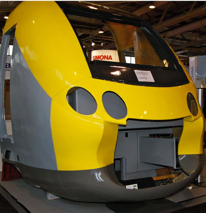
LEFT: A driver's cab mock-up made from composites by NewRail to demonstrate the possibilities of the material
