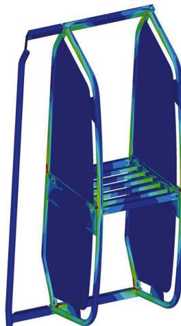
RIGHT: A simulation conducted by Siemens to test a baggage rack
