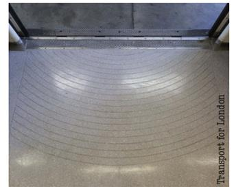
**L**ondon Underground transports approximately 1.3 billion passengers every year and so a heavy-duty floor covering is essential – and it also fulfills a critical safety role. The most recent project undertaken by Treadmaster for London Underground involves the supply of more than 9,000m<sup>2</sup> of its TM7 flooring product for the refurbishment of 36 seven-car metro trains (built in 1972) on the Bakerloo line.
