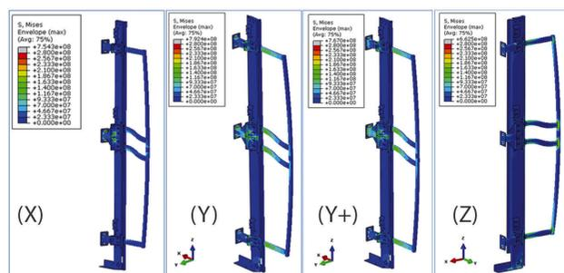
ABOVE: Stress simulations conducted by Integral for Metrovagonmash in the course of developing a handrail for the Moscow Metro
