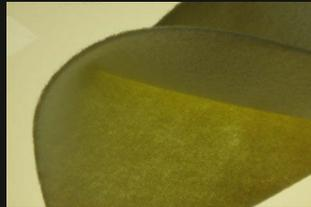
The custom-engineered spun-laced and needle-punched materials offered by Norafin are suitable for use as fire blockers in a range of markets, including public transport. Norafin says these technical non-woven materials' fire blocking and fire retarding capabilities accord with EN 45545-2, FAR/CS25.853a, ABD 0031-F and BSS 7239 standards, and the materials also comply with railway standards regarding the emission of smoke and toxic gases.
